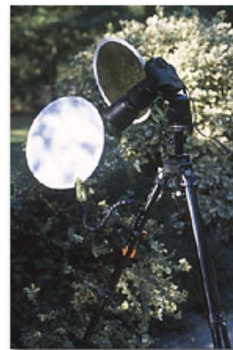
Wimberley Plamps are ideal for securing the LiteDiscs to the tripod legs and holding the discs in position.
