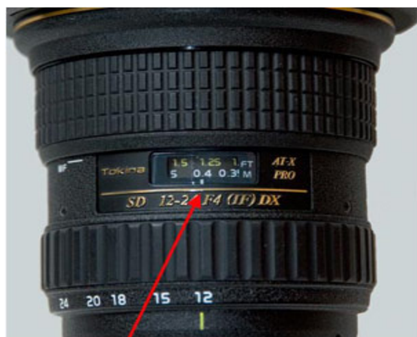
Hyperfocal point for 12mm at f/22 (1.3'/.4m). Focus point obtained from hyperfocal chart.
