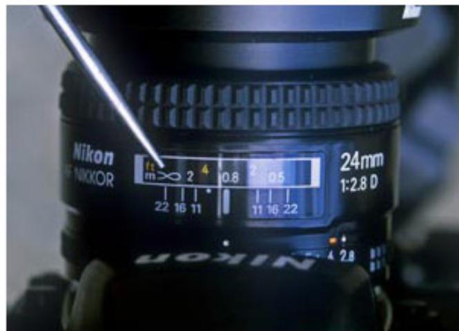
Setting the hyperfocal point on a fixed focal length lens.
