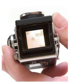
With the hood opened on top of the camera, the viewing LCD can be seen. To close the hood, pinch the sides of the hood inward to collapse the hood and close the cover.
