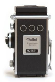
The back of the camera has a row of three buttons that are used for viewing the photos on the SD card and for setting resolution. Facing the back of the camera from left to right; Image delete button, Previous image, Next image. When in Record mode, the Previous and Record buttons are also used for setting resolution. In the viewfinder, H equals 1760 X 1760, N equals 1200 X 1200 and L equals 640 X 640. Please keep the camera set at the highest (H) resolution!
